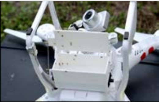
Tiny biocontrols for water hyacinth and other invasive plants are housed and delivered to vegetation via a vertical-takeoff quadcopter.
