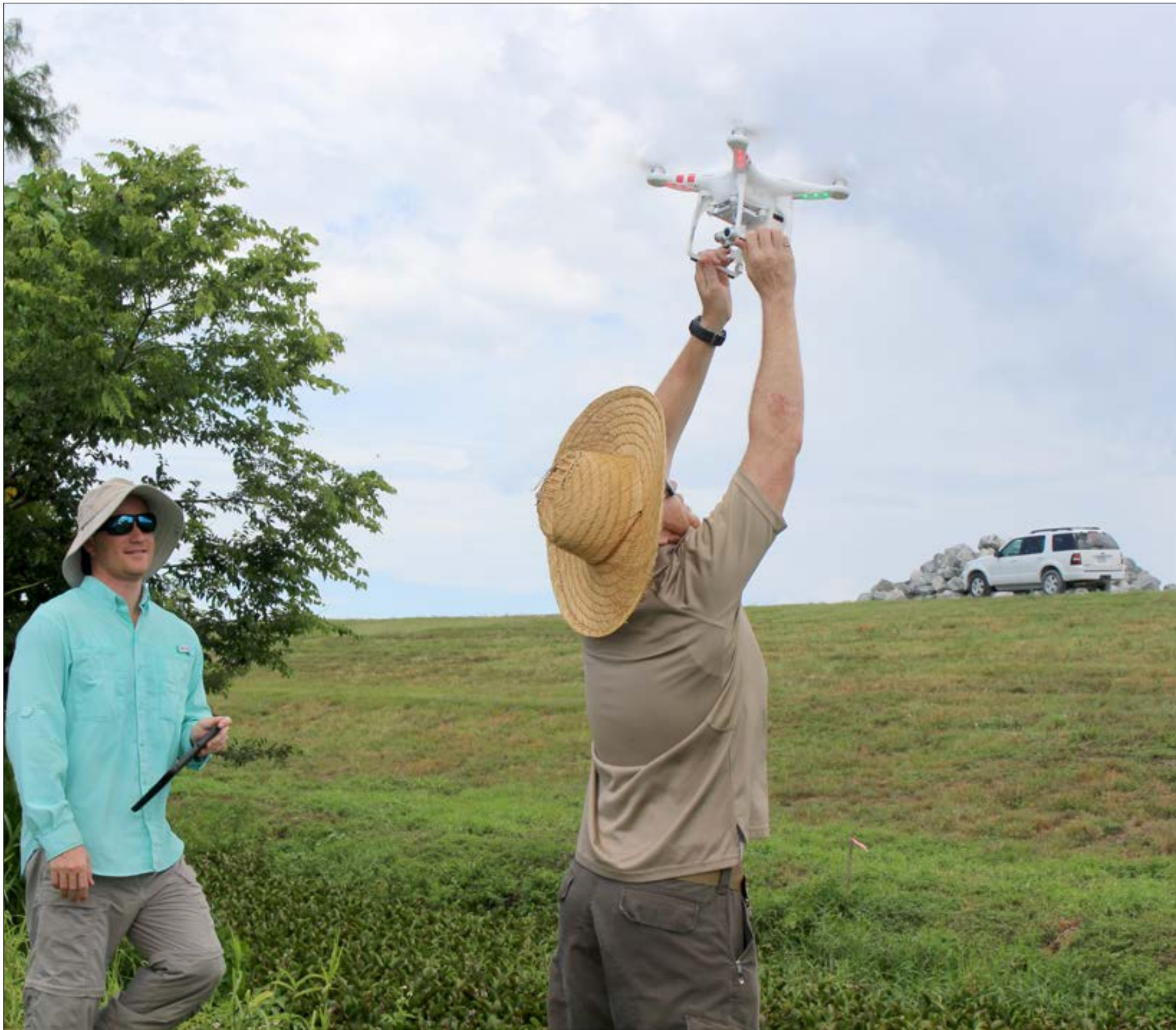
Thomas Spencer engineered an innovative solution to deliver biocontrol organisms to areas previously inaccessible to invasive species managers, such as tree canopies and remote wetland locations. Victor Wilhem releases the specially-outfitted vertical lift quadcopter with a remotely operated drop box and camera to monitor and confirm delivery in real time.
