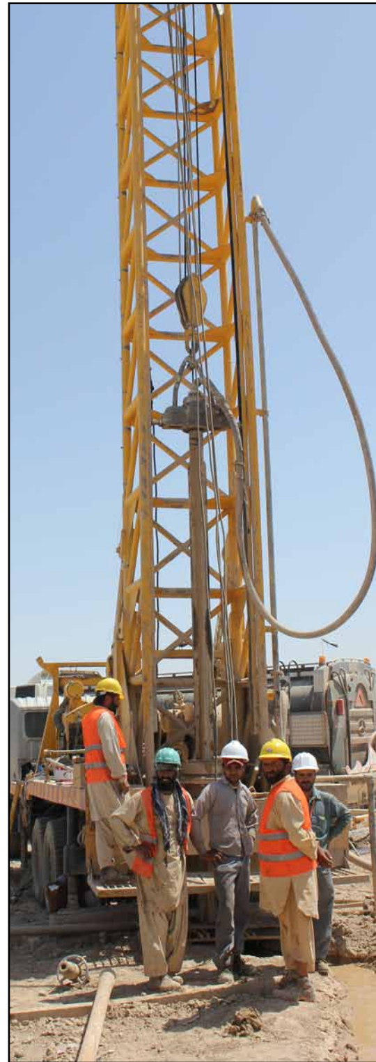
An example of a modern Afghan well-drilling rig with a trained crew. The crew just hit good quality water at a depth of 420 meters. (Photo by Len Sinfield)
