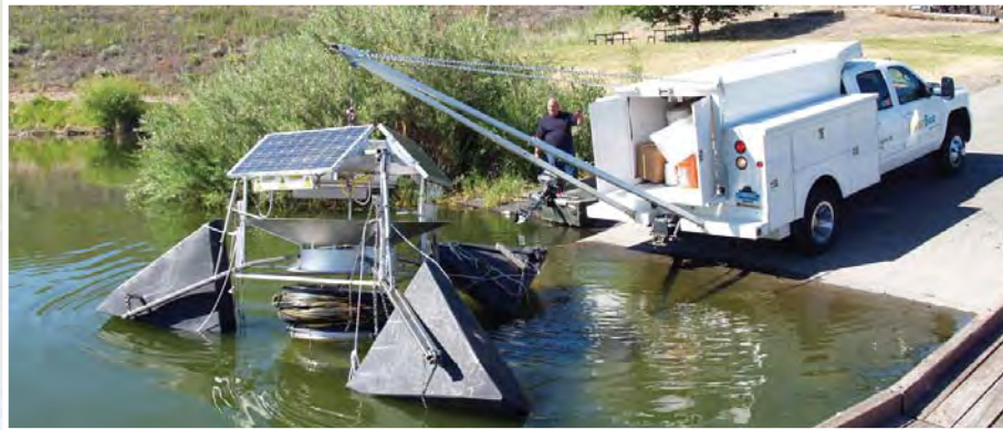
One of two solar-powered long-distance circulators is placed into Willow Creek Reservoir in Oregon as part of a pilot study to manage harmful algae blooms. The unit draws water from a specified depth and distributes it throughout the reservoir. This process mixes the specified layer of reservoir, disrupting blue-green algal habitat.
