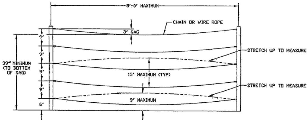
MARINE TYPE C NON-TENSIONED RAILING (3" SAG SHOWN)
