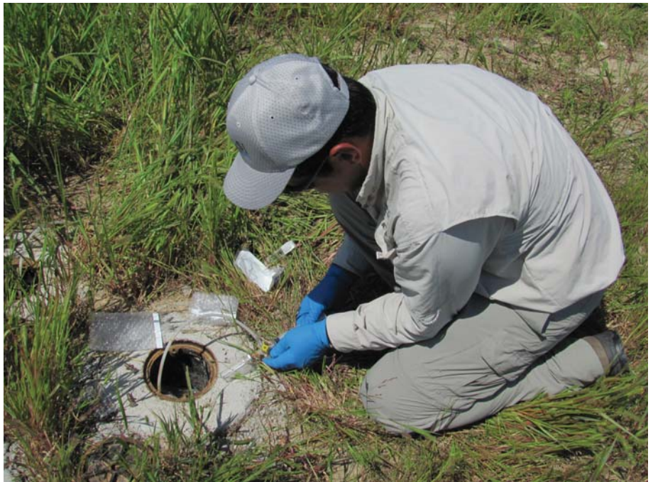
Ahmad Seyedabbasi, of GSI Environmental Inc., performs soil gas sampling at one of the vadose zone monitoring point locations. (Photo by Charles Coyle)
