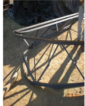
Picture of the buckled bar joist
