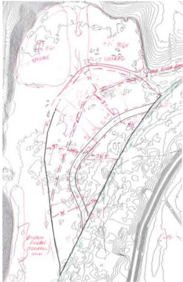
Figure 3.3-4. Initial design drawings of the Channel Overbank Flooding Natural Scour Alternative
