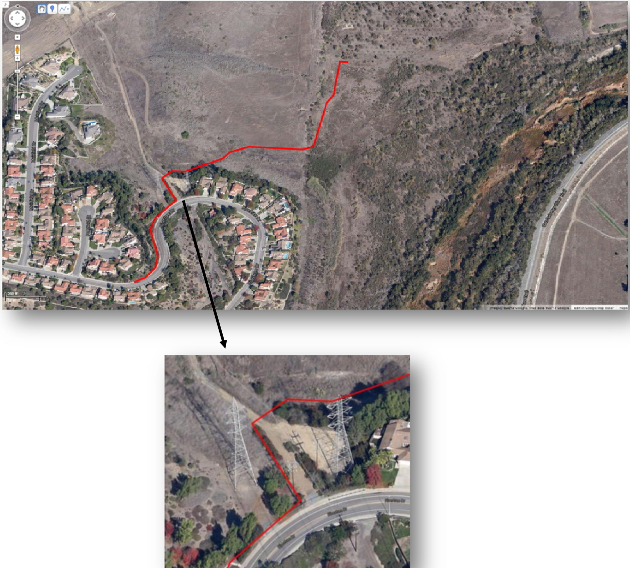
Figure 3.3-9. Irrigation mainline alignments to restoration site passing through undeveloped open space to minimize disturbance to the nearby community and paved roads
