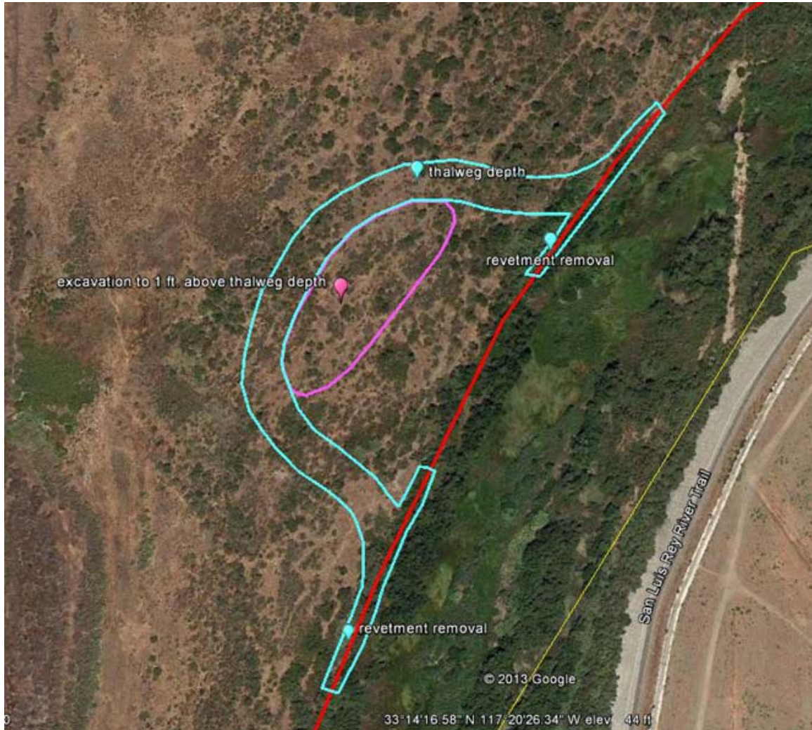
Figure 3.3-2. Natural scour alternative design
