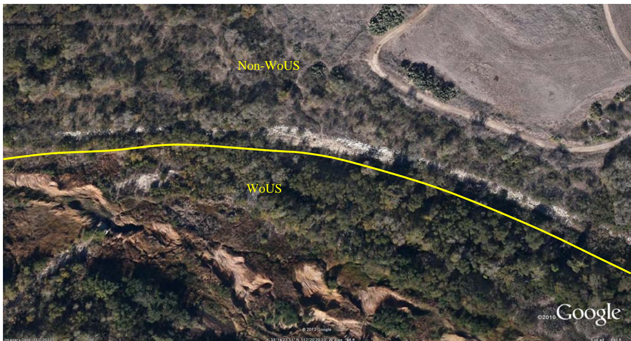
Figure 2: Representative aerial view of a portion of the mitigation site showing the lateral extent of waters of the United States based on a distinctive vegetation boundary between mulefat (FAC) and cattails (OBL) species
