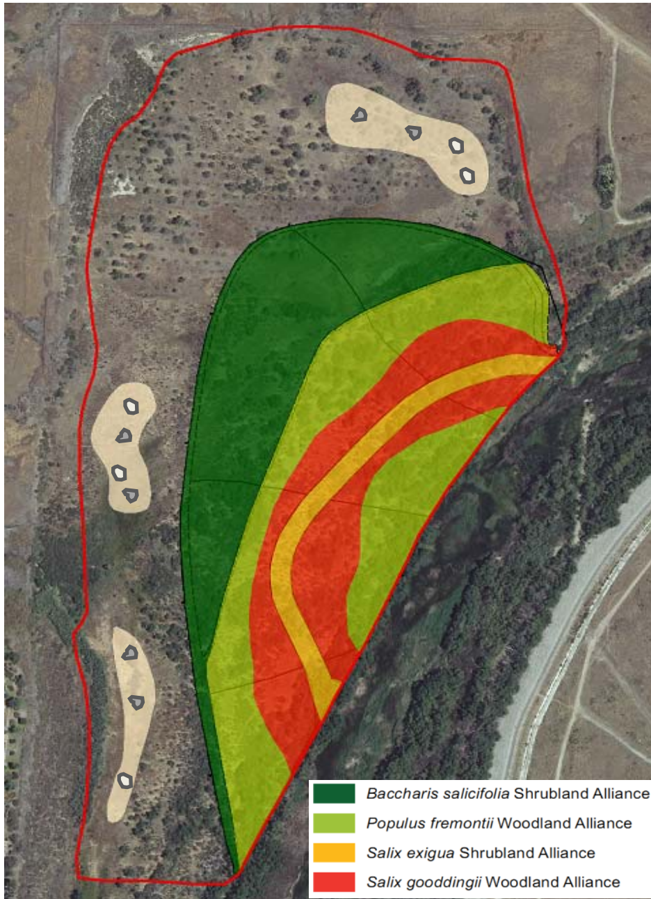
Figure 3.3-5. Vegetation type alliances being restored along with three soil disposal sites that will be compacted to approximately 80%-85%, hydroseeded with coastal sage scrub seed mix, and rock rubble mounds placed onto top for ground squirrel and burrowing owl habitat.
